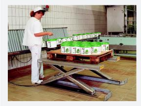
The stainless steel EdmoLift TUB 1000 lifting table is a superlow table, ready for operation without the need for pit mounting. The pallet can be loaded directly on to the U-shaped platform with a hand pallet truck.
