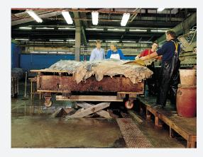
Heavy lifting and bad working postures are common place in tanneries. The image shows a stainless steel lifting table which provides good ergonomic working practices whilst resisting the harsh affects of tannic acid, a much needed help in the tanning process. An investment in a EdmoLift lifting table is both rational and cost effective. It prevents wear and tear on the body of the operator and reduces absenteeism.
